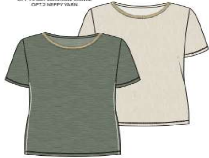
METALLIC NECK TRIM & S/SEAM CHAIN STITCH EMBROIDERY OPT.1. POLY ELASTANE CRINKLE OPT.2 NEPPY YARN
